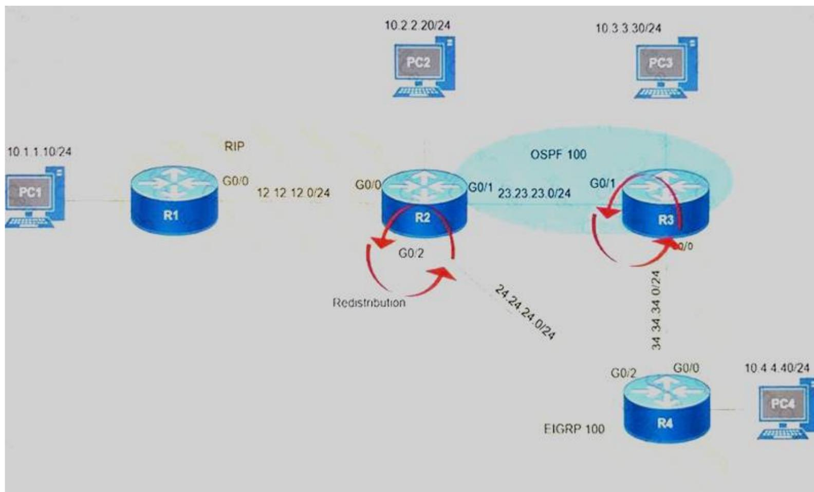
After redistribution is enabled between the routing protocols; PC2, PC3, and PC4 cannot reach PC1. Which action can the engineer take to solve the issue so that all the PCs are reachable?
