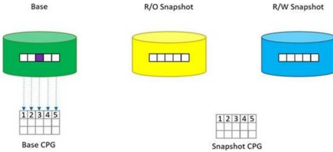
You create two snapshots of a thin provisioned base volume in an HPE Primera. One snapshot is read only and the other is read-write. A write occurs at the location shown in in the diagram.
