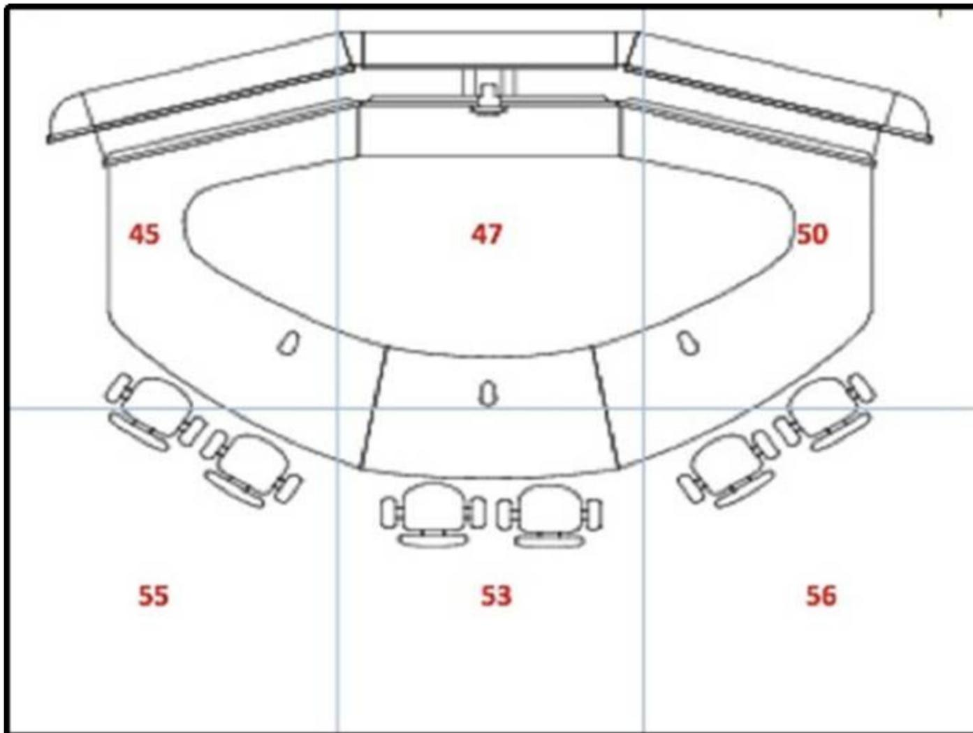
Acoustic measurements for ambient noise were taken on a candidate for an Immersive Cisco TelePresence room. The numbers on the floor plan represent the dBA readings for each of the six areas of the room.
