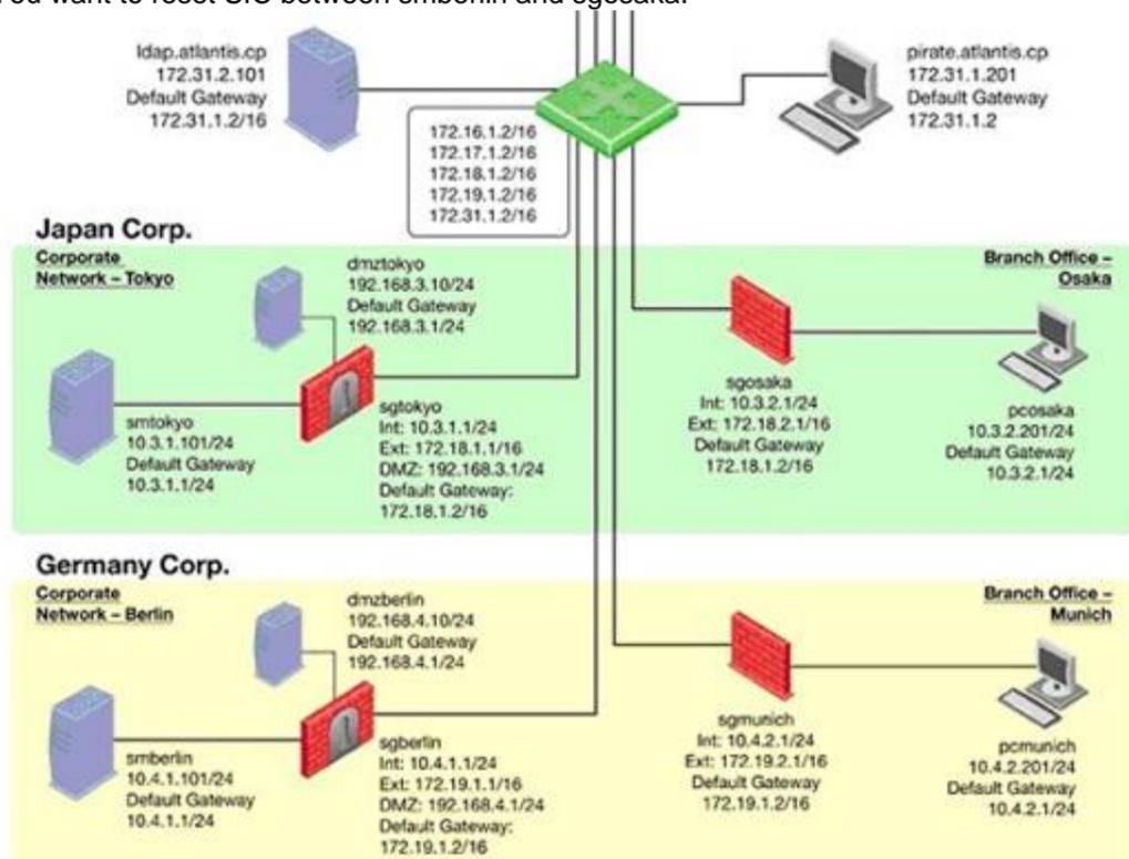
In SmartDashboard, you choose sgosaka, Communication, Reset. On sgosaka, you start cpconfig, choose Secure Internal Communication and enter the new SIC Activation Key. The screen reads The SIC was successfully initialized and jumps back to the cpconfig menu. When trying to establish a connection, instead of a working connection, you receive this error message:
