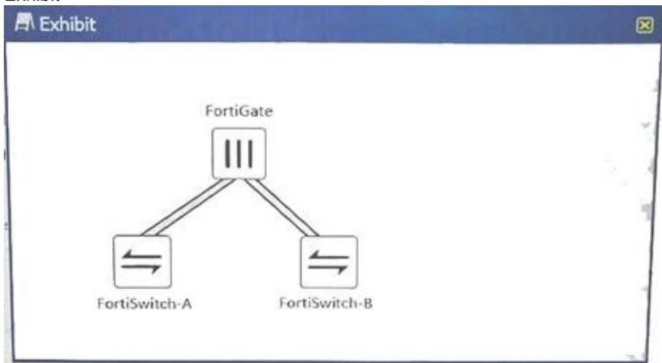
An administrator implements a multi-chassis Link aggregation (MCLAG) solution using two FortiSwitch 448Ds and one FortiGate 3700D. As described in the topology shown in the exhibit, two links are connected to each FortiSwitch. What is required to implement this solution? (Choose two)
