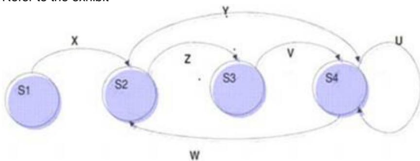
Given the following State Transition diagram, match the test cases below with the relevant set of state transitions.
