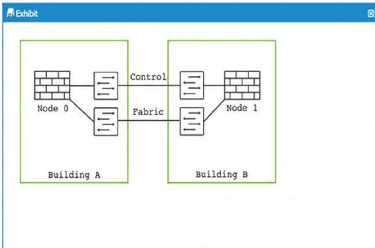
You are designing a security solution using an SRX Series chassis cluster in two separate buildings. In this scenario, what are three considerations? (Choose three)
